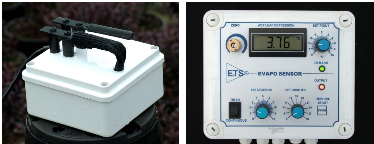
Fig. 1 The Evaposensor (left) has now moved from being a research tool to having full commercial application thanks to the development of a versatile control interface (right) from E&TS Ltd.
